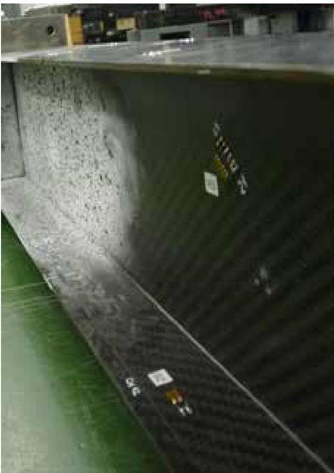
Figure 12: The beam after the test with no visible residual deformation
