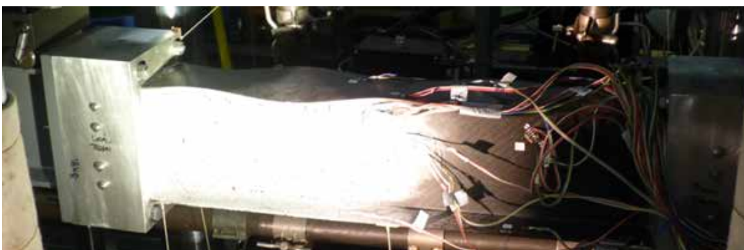
Figure 9: Buckling of the upper flange buckling from front side.
