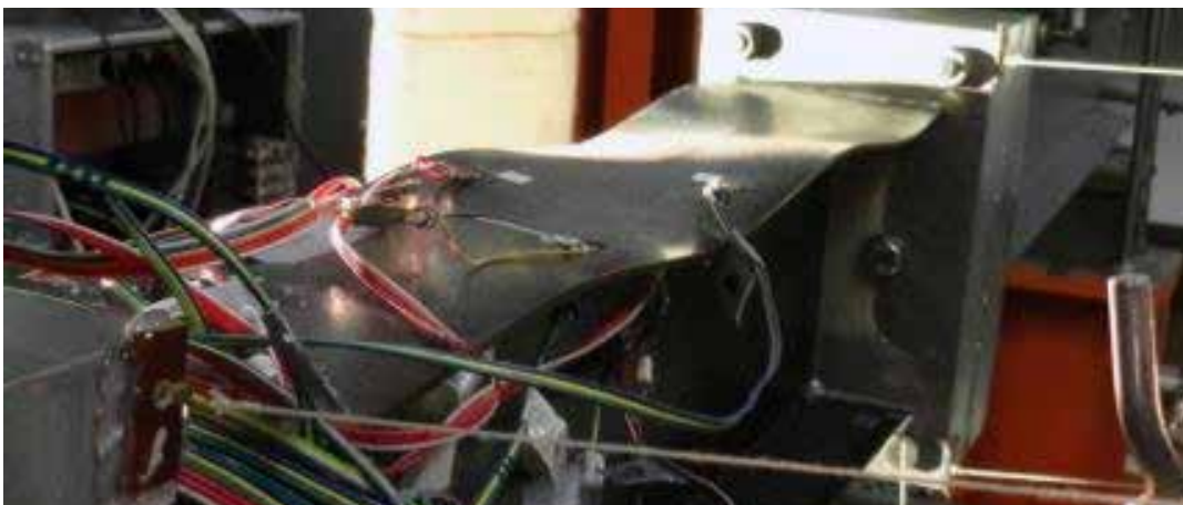
Figure 11: Buckling of the upper flange at maximum load.
