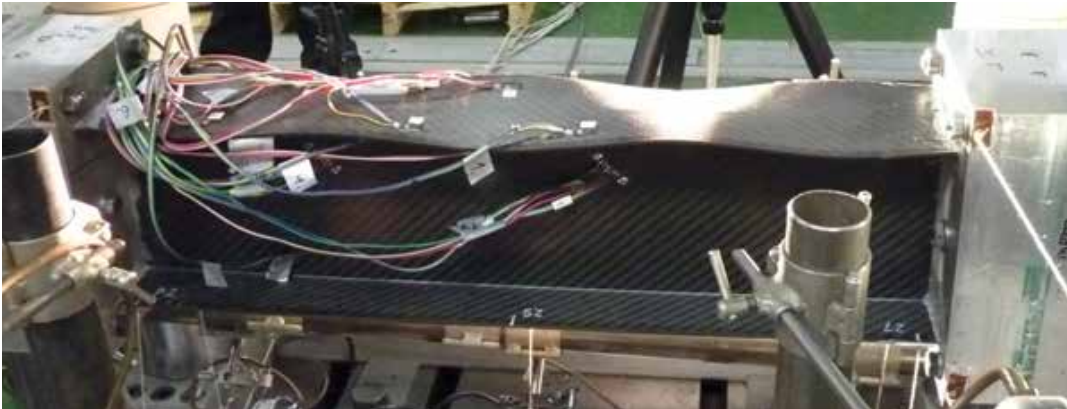
Figure 10: Buckling of the upper flange from rear side. Symmetrical mode with 5 local extremes is visible.
