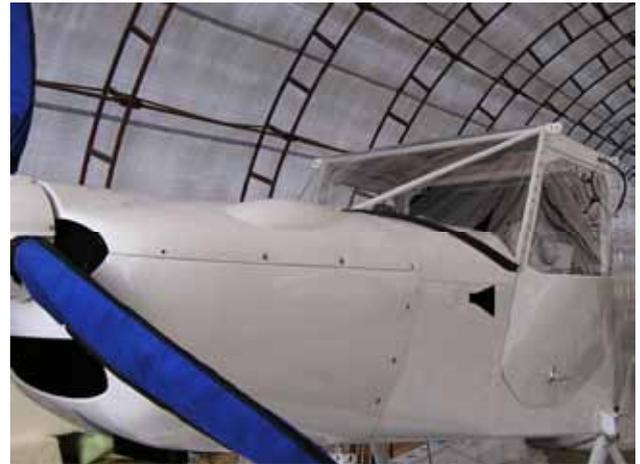
Fig. 8 Engine hood of ultralight CHS 701SP – prototype
