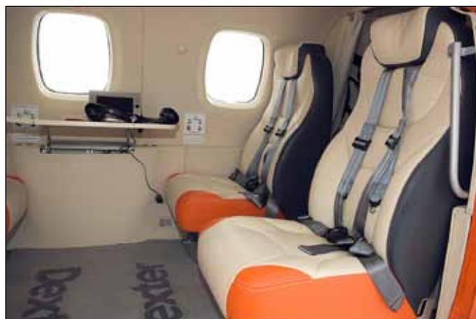
Fig.12 Interior panels of M101 Expedition made by LF Technology with LFX 038 according to FAR 23
