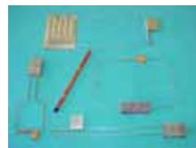
Fig. 2 Miniature LHPs with cylindrical evaporators
