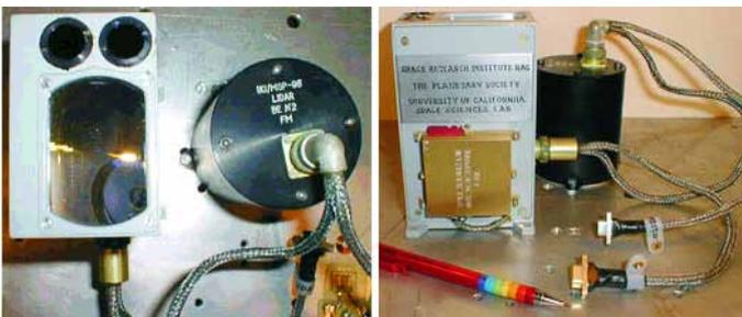
**Fig. 1: The flight unit of lidar on MPL'98. Optical part (silver block with apertures) with two lasers and receiver; and electrical part (black cylinder).**
