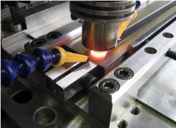
Fig. 4 – FSW of stainless steel profile in VZLU
