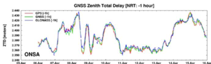
Fig. 6 ZTD time-series based on multi-GNSS and stand-alone GPS and GLONASS solutions by GOP
