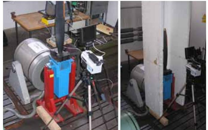
Fig. 1: Composite propeller blade mounted in a special fixture for excitation of the first three natural vibration modes. The thermograms were taken using a thermal insulating box.
