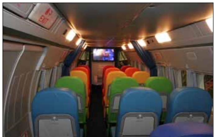
Fig. 16 LF Technology was used for the production of the ceiling interior panels in airplane L-410 (according FAR 23)
