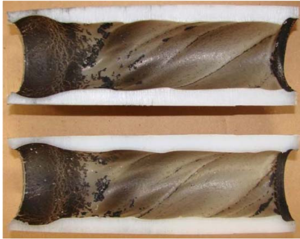
Figure 2 - Swirl oxidizer injector, model 1
