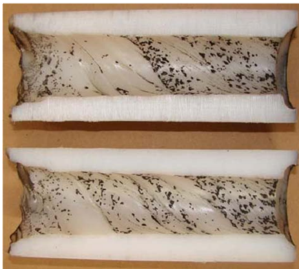
Figure 4 - Swirl oxidizer injector, model 2
