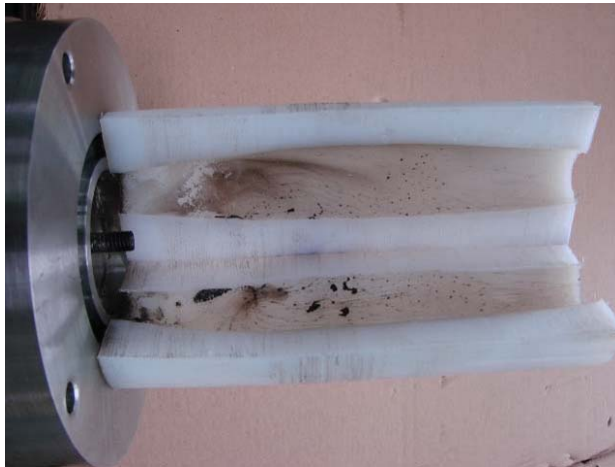
Figure 3 - Axial oxidizer injector
