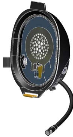
Figure 2 - Active Noise Reduction module inside personal headset
