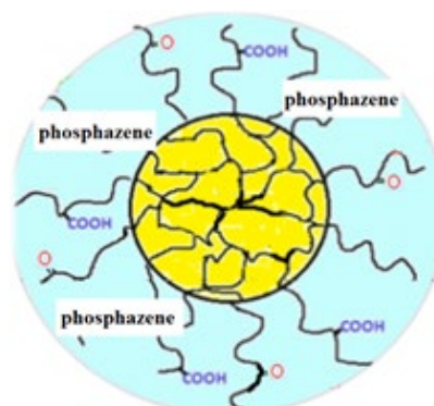
Figure 2 - Latex particles core-shell structure
