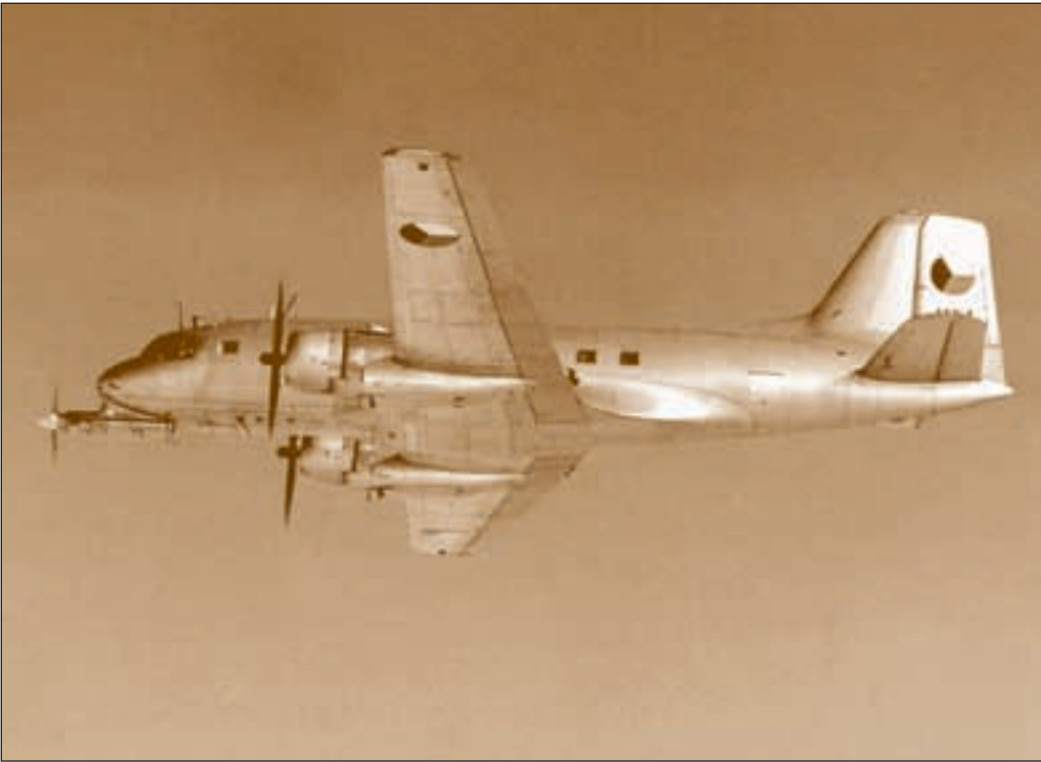
First flight of M-601/V-508 power plant mounted on IL-14 flying lab on 24 November 1969
