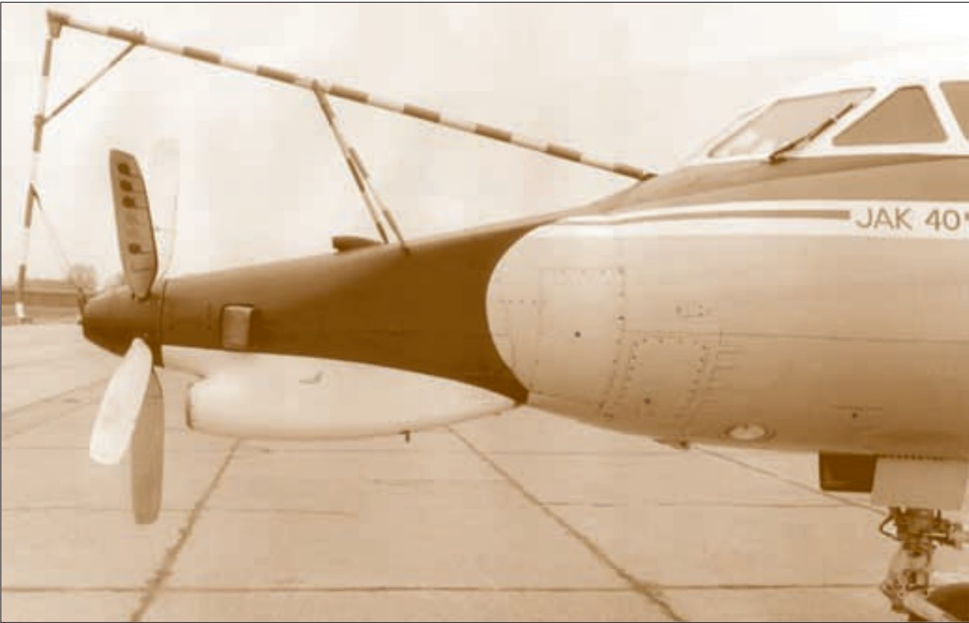
YAK-40 flying lab with device for strain gauge testing of V-510 propeller
