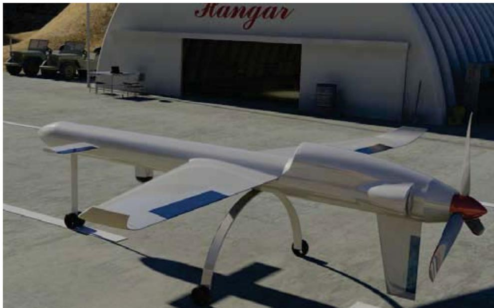
Autodesk Inventor into Autodesk 3ds Max Design, the default settings of surfaces and the import itself worked without any problem, i.e. the number of surfaces was sufficient for the complex shapes of individual engine parts. This was followed by setting the model in motion, texturing, lighting, camera setting and image and animation rendering proper.
